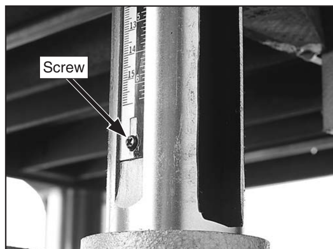
Figure 46. Location of adjustment screw for table elevation scale.
