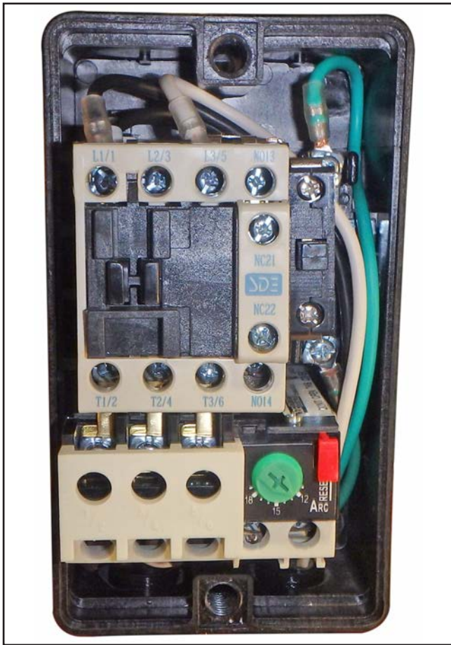
Figure 53. G0890/G0891 magnetic switch with cover removed.
