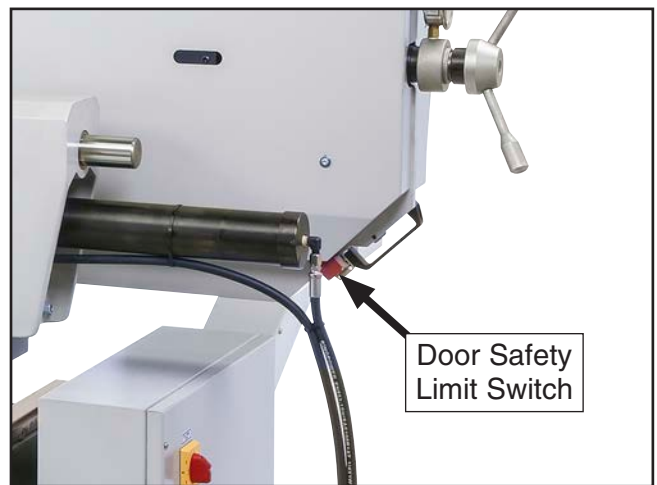
Figure 132. Door safety limit switch.
