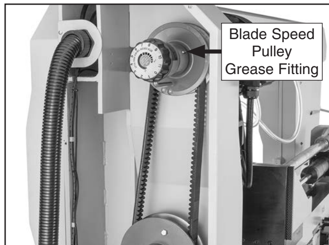
Figure 76. Blade speed pulley grease fitting location.
