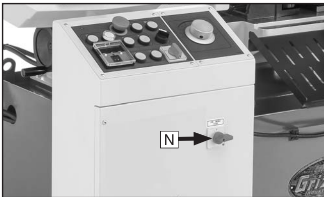
Figure 2. Master power switch location.
