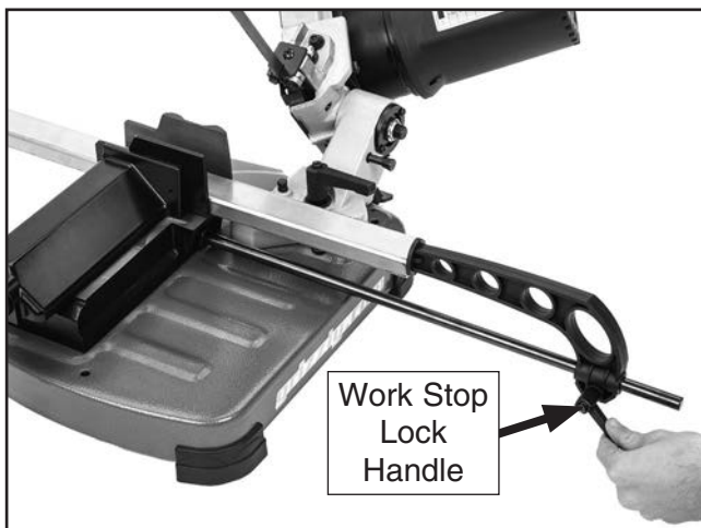
Figure 22. Setting work stop to support repetitive cutting operation.
