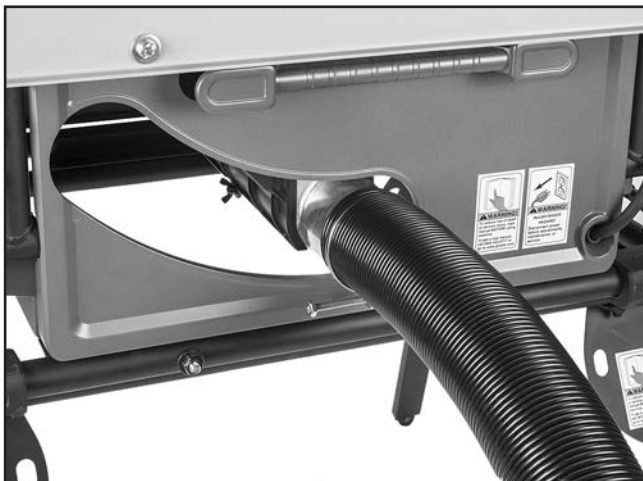
Figure 21. Dust hose attached to dust port.
