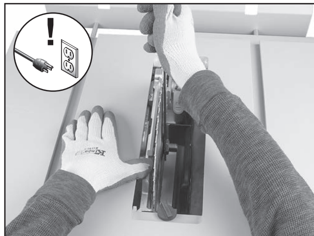
Figure 30. Example of removing table saw blade.
