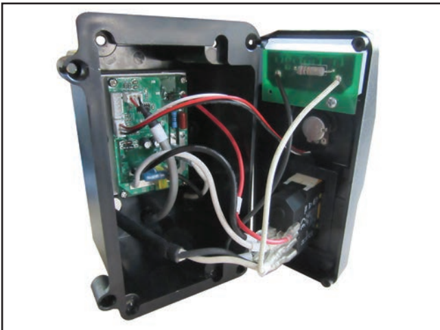
Figure 92. Wiring junction box with cover removed.
