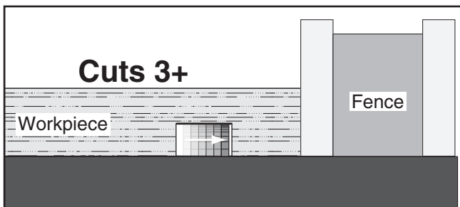
Figure 49. Additional single-blade dado cuts.
