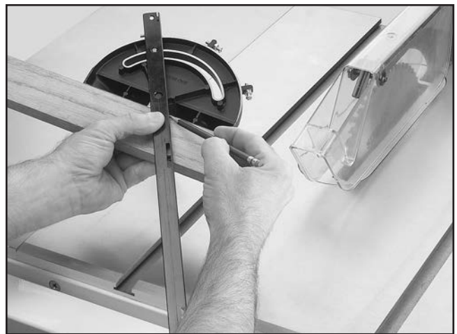
Figure 43. Example of marking miter line.
