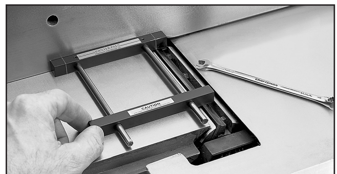
Figure 35. Setting knife height with a Jointer Pal®.
