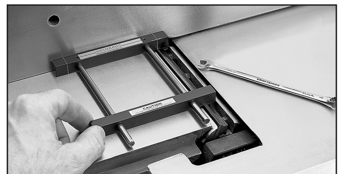
Figure 35. Setting knife height with a Jointer Pal®.
