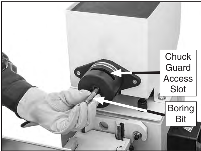
Figure 16. Removing bit from chuck.
