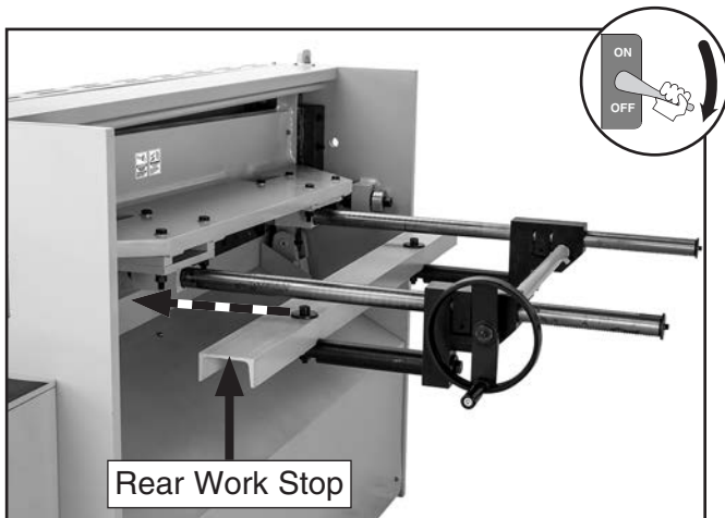
Figure 66. Checking rear work stop parallelism.
