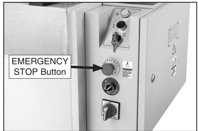
Figure 28. Control panel EMERGENCY STOP button.
