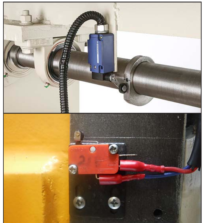
Figure 77. Blade travel limit switch (top) and blade guard limit switch (bottom).
