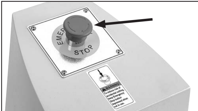
Figure 27. Foot pedestal EMERGENCY STOP button.
