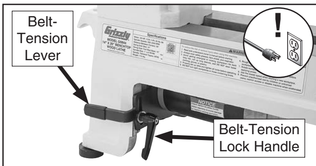
Figure 42. Belt tension controls.
