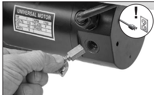
Figure 48. Removing brush from motor.
