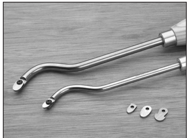
Figure 41. Swan neck hollowing tools.
