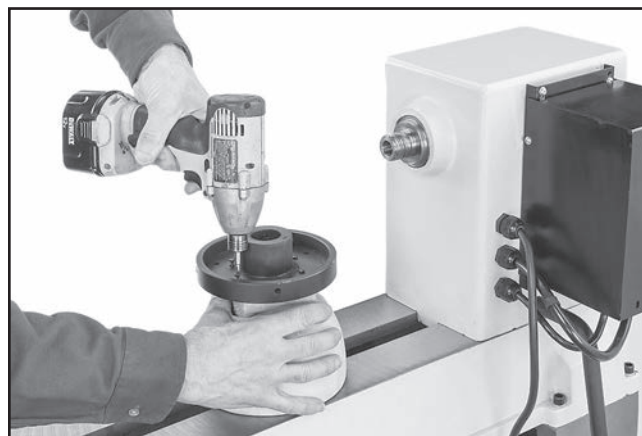
Figure 32. Typical attachment of faceplate to workpiece.
