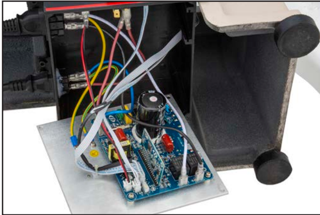
Figure 49. Control box wiring.
