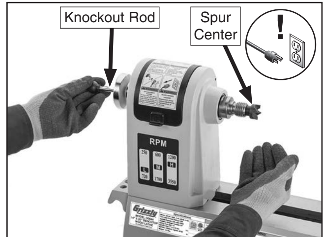
Figure 17. Example of removing headstock center with knockout rod.
