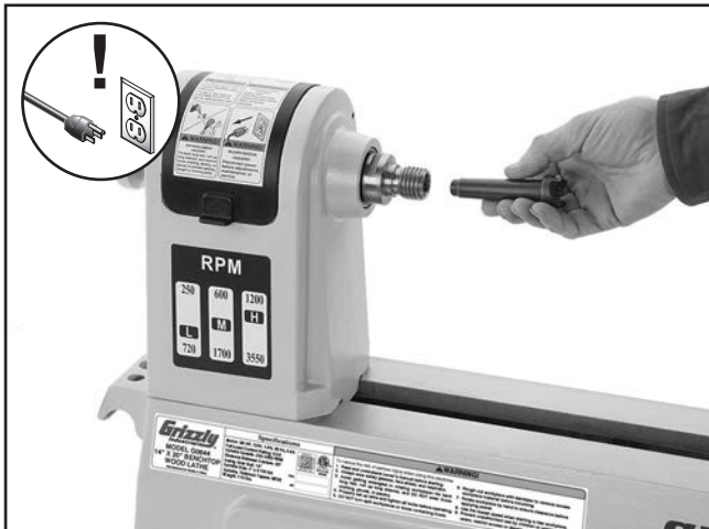
Figure 16. Example of installing center in headstock spindle.
