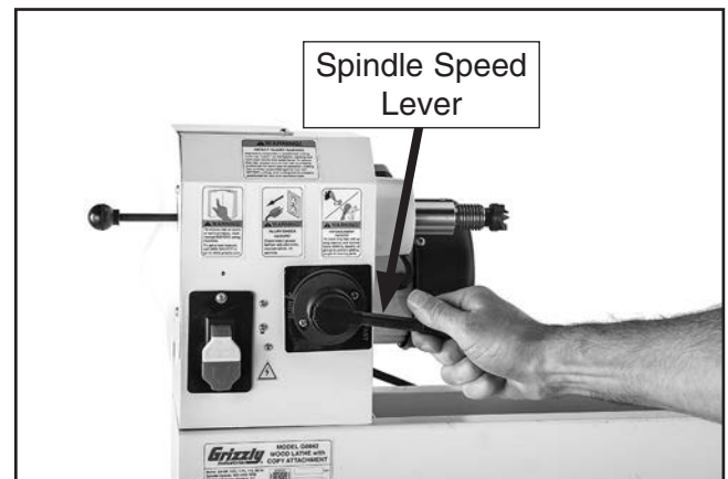
Figure 62. Spindle lever turned right.
