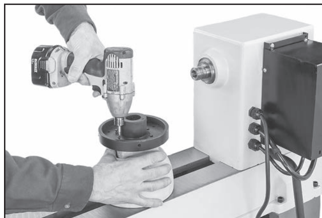
Figure 48. Typical attachment of faceplate to workpiece.
