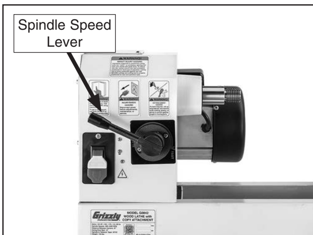
Figure 41. Spindle speed shift lever shown at low setting.
