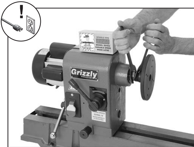
Figure 40. Example of tightening faceplate onto spindle.
