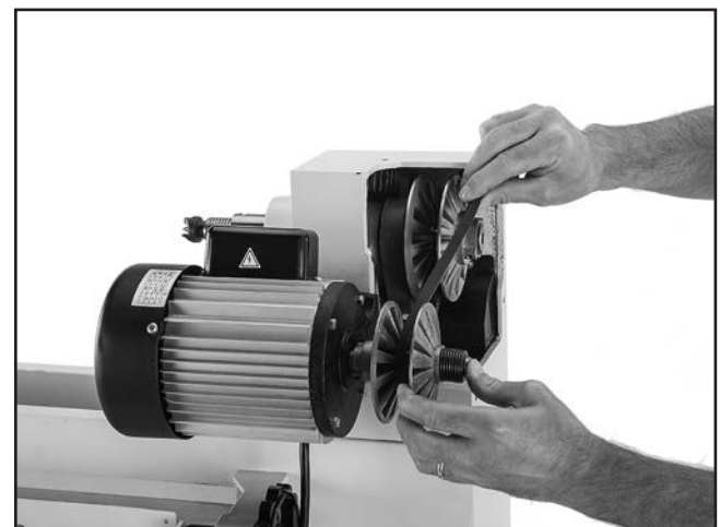
Figure 63. Removing V-belt from spindle pulley.
