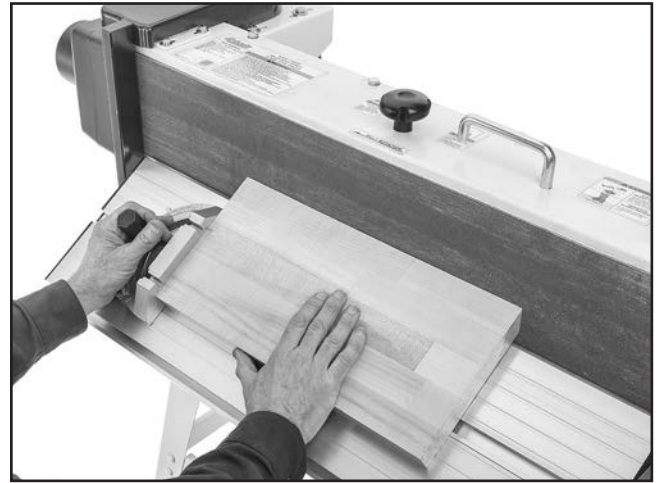
Figure 39. Example of edge bevel sanding with miter gauge.
