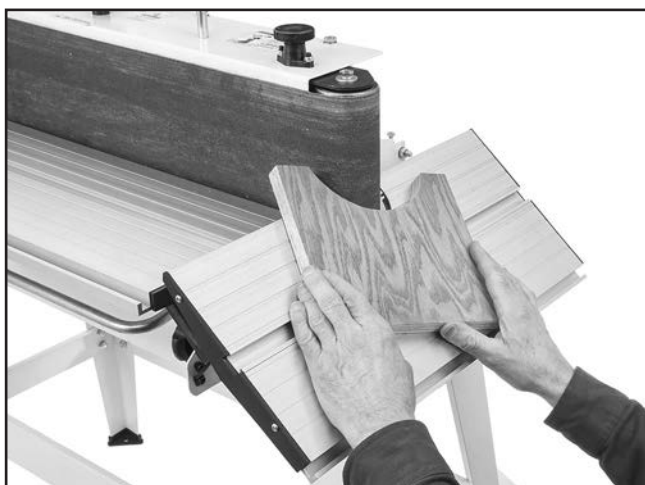
Figure 41. Example of contour bevel sanding.
