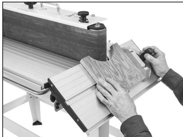
Figure 42. Example of contour bevel sanding with miter gauge.
