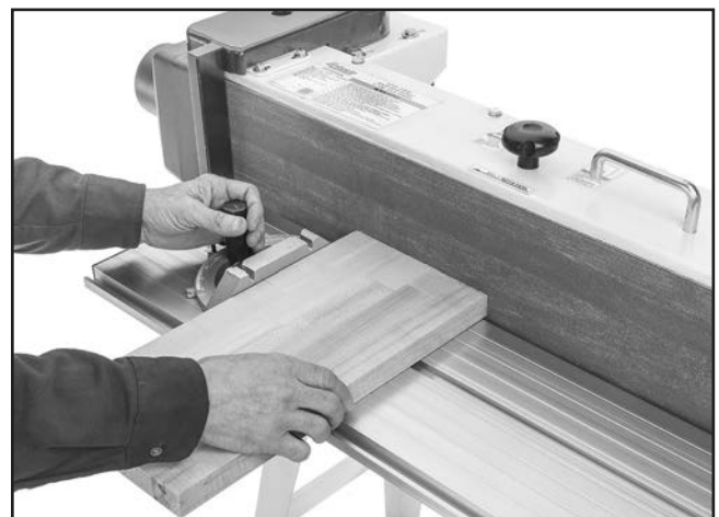
Figure 35. Example of end sanding.
