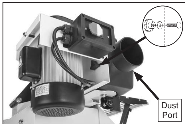
Figure 20. Dust port attached to edge sander.
