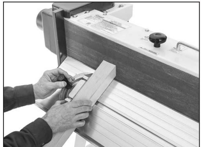
Figure 40. Example of end bevel sanding with miter gauge.
