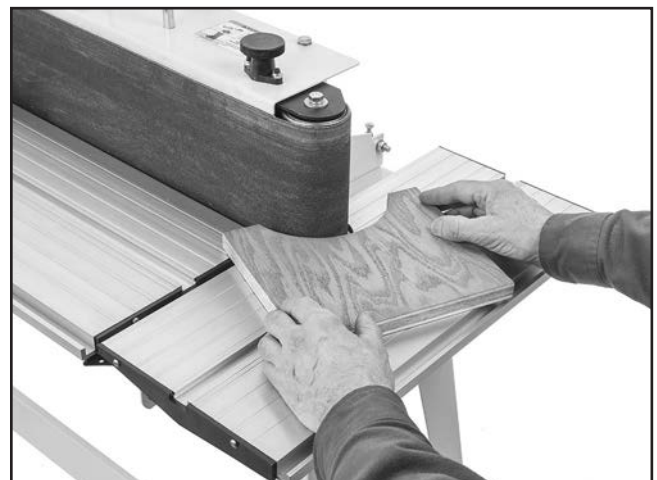
Figure 37. Example of contour sanding.
