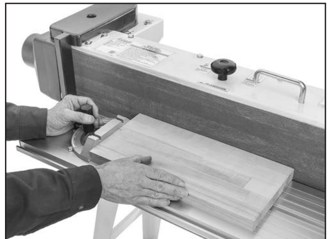
Figure 34. Example of edge sanding with miter gauge.
