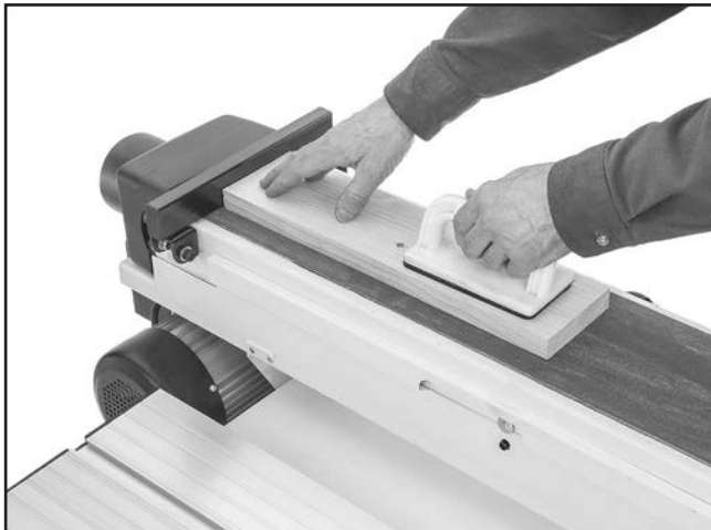
Figure 36. Example of face sanding.
