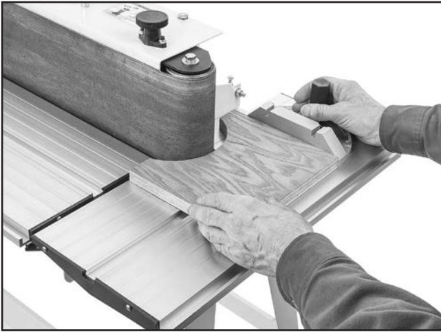
Figure 38. Example of contour sanding with miter gauge.
