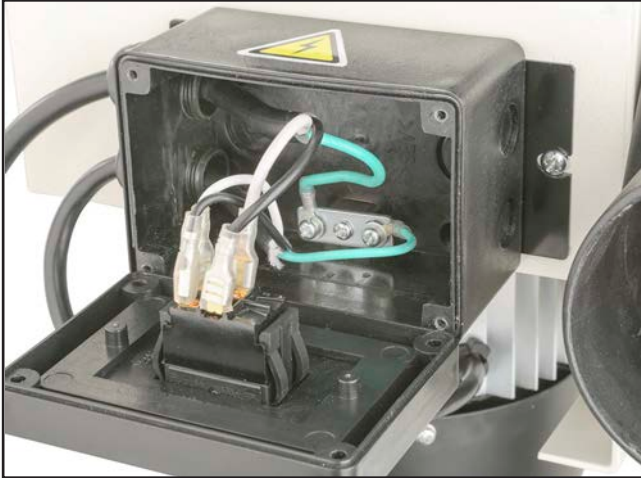
Figure 58. G0839P switch box and connections.
