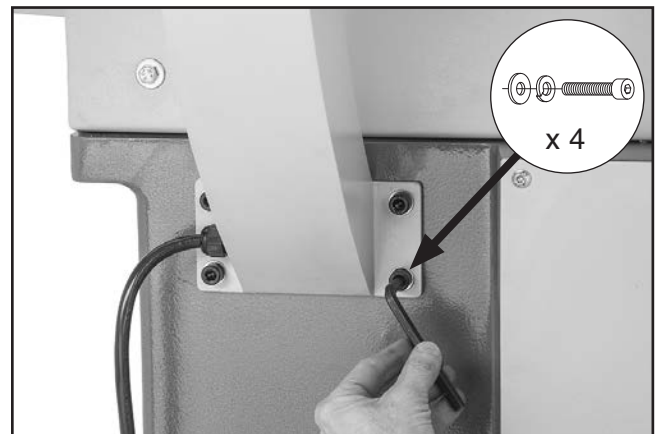
Figure 15. Securing control panel pedestal.
