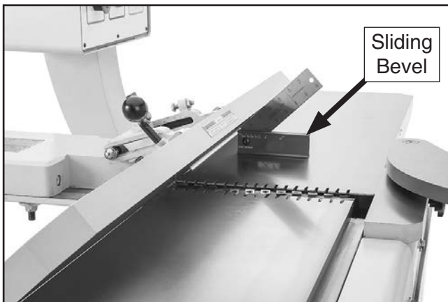
Figure 62. Adjusting fence to 45° inward.
