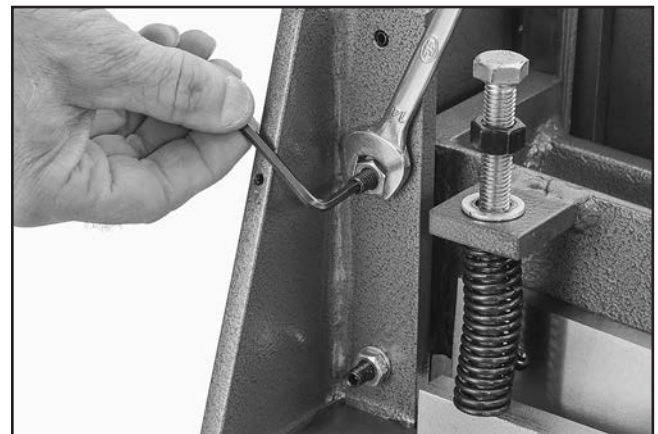
Figure 40. Tightening gib set screw.
