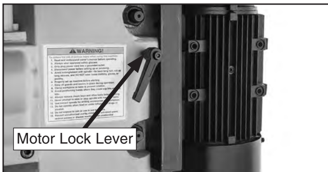
Figure 16. Use lock lever when changing V-belt positions to change spindle speed.
