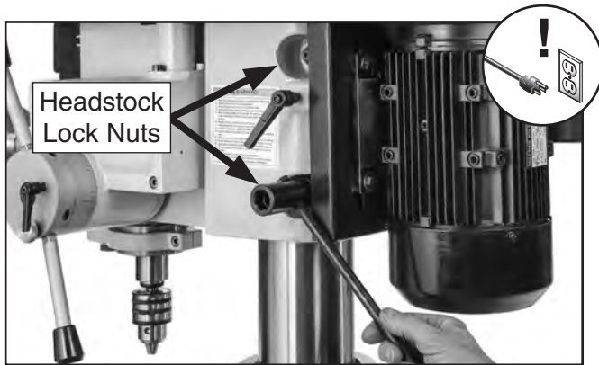
Figure 23. Loosening headstock lock nuts in order to adjust headstock position.
