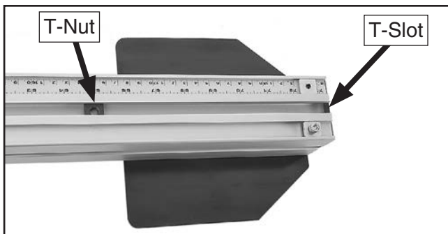
Figure 48. T-nut installed on right end of crosscut table T-slot.
