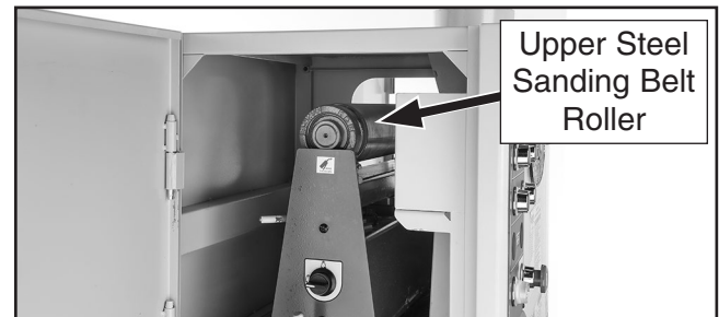
Figure 13. Steel sanding belt roller that must be cleaned thoroughly before using machine.
