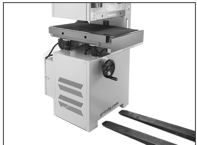
Figure 17. Lifting machine with forklift.
