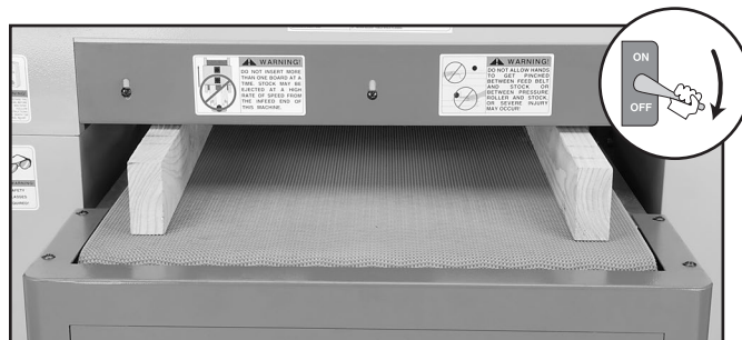
Figure 75. Example of 2x4s placed on conveyor belt under sanding drum.
