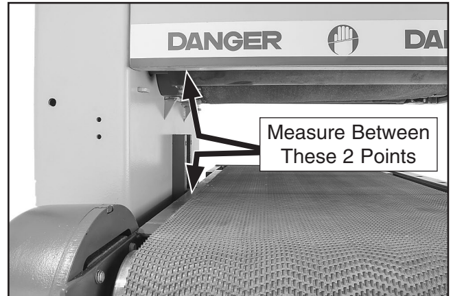
Figure 71. Rear right measurement location for checking table parallelism.
