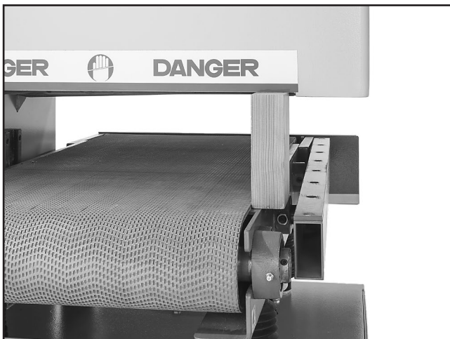
Figure 70. Position of wood block on conveyor table.
