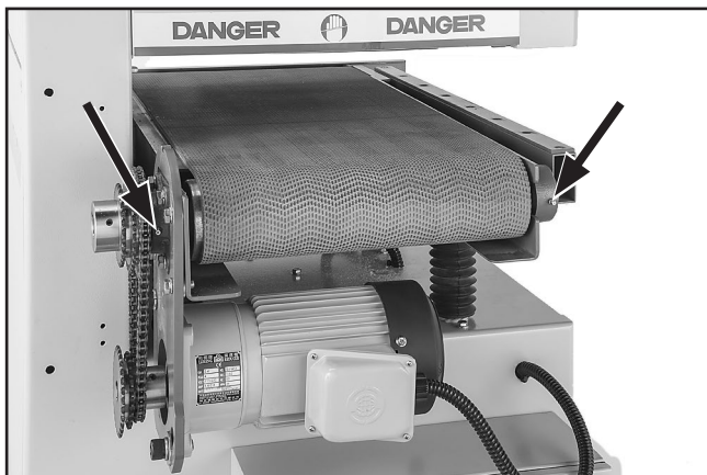
Figure 48. Locations of conveyor belt roller axle grease fittings (chain cover removed for access).
