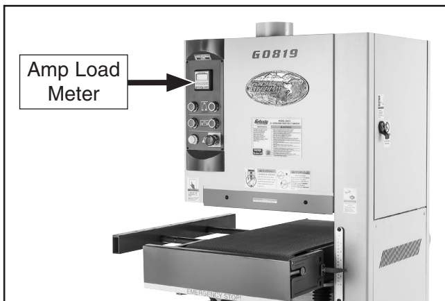
Figure 34. Location of amp load meter.
