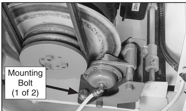
Figure 60. Location of disc brake assembly mounting bolts (1 of 2 shown).
