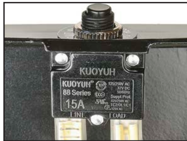
Figure 100. Main motor circuit breaker wiring.
