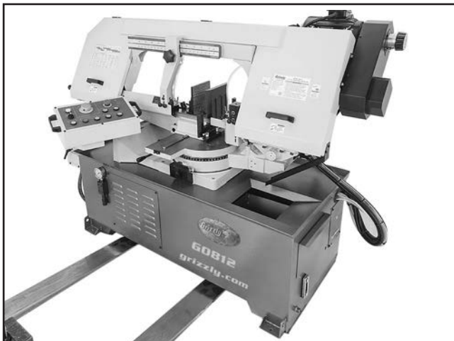
Figure 10. Inserting forklift forks for lifting machine.
