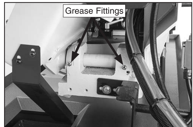
Figure 69. Pivot-point grease fitting locations.
