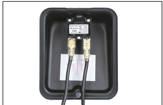
Figure 67. Circuit breaker wiring.
