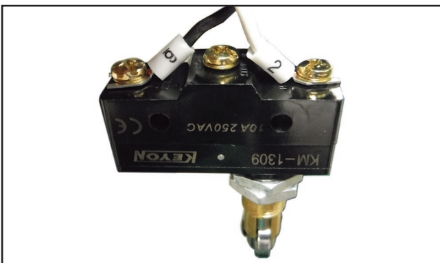
Figure 65. Limit switch wiring.
