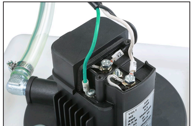
Figure 68. Coolant pump wiring.
