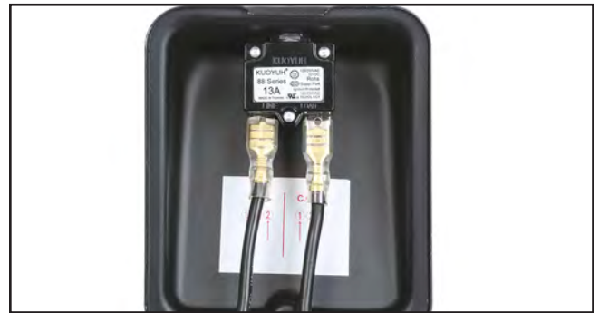
Figure 68. Circuit breaker wiring.
