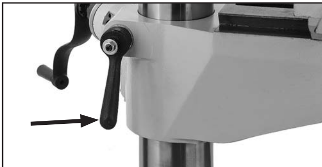
Figure 17. Location of Z-axis table lock.
