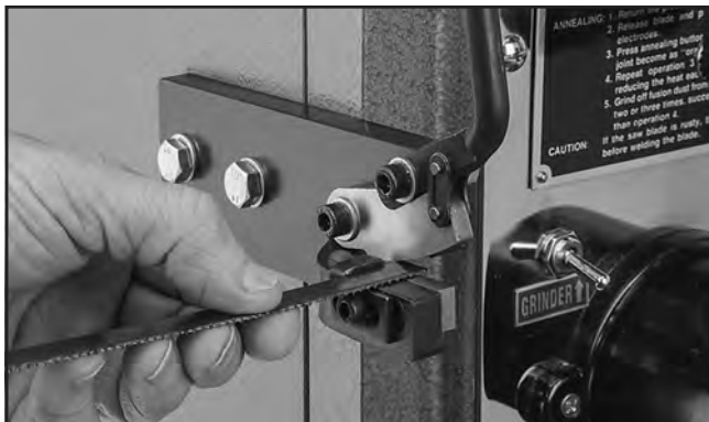
Figure 43. Using the blade shear to cut the blade.
