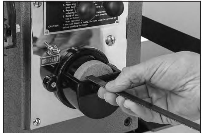
Figure 44. Using the grinder to square up the blade end.
