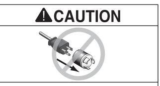
No adapter should be used with plug. If plug does not fit available receptacle, or if machine must be reconnected for use on a different type of circuit, reconnection must be performed by an electrician or qualified service personnel, and it must comply with all local codes and ordinances.
