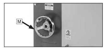
Figure 2. Variable-speed handwheel.
