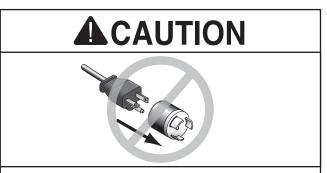
No adapter should be used with plug. If plug does not fit available receptacle, or if machine must be reconnected for use on a different type of circuit, reconnection must be performed by an electrician or qualified service personnel, and it must comply with all local codes and ordinances.
