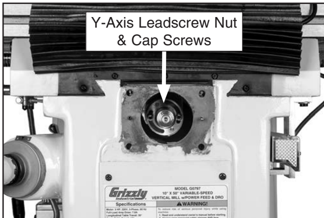
Figure 85. Y-axis leadscrew nut and cap screws.
