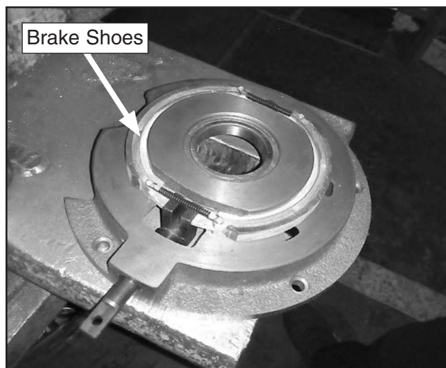
Figure 106. Lower pulley, shaft, and bearing sleeve removed to expose brake shoes for inspection/replacement.
