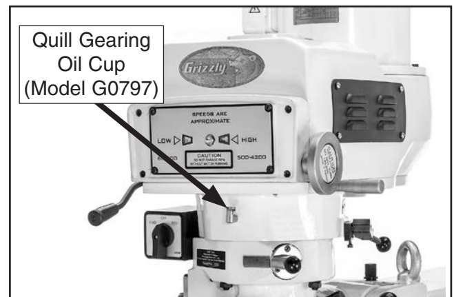
Figure 69. Location of Model G0797 quill gearing oil cup.
