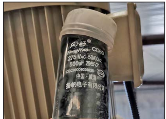
Figure 109. Run and start capacitors.
