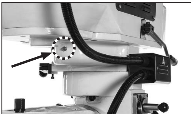
Figure 71. Model G0797 headstock gearing grease fitting.
