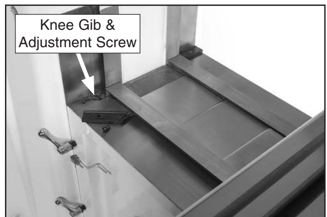
Figure 81. Knee gib and adjustment screw.
