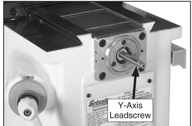
Figure 83. Ball handle, ring, and key removed from Y-axis leadscrew.
