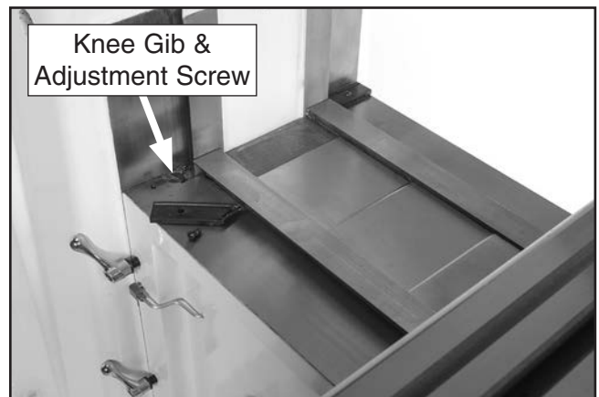
Figure 81. Knee gib and adjustment screw.
