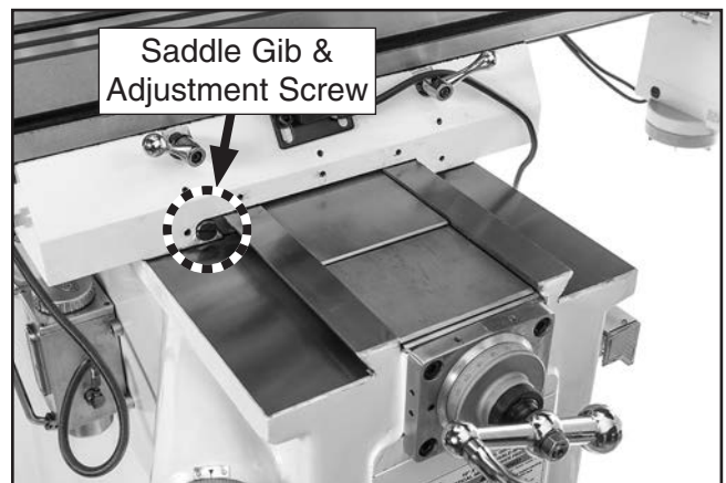
Figure 80. Saddle gib and adjustment screw.
