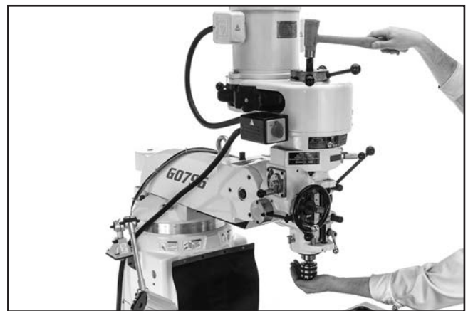
Figure 54. Tapping drawbar to unseat tool taper (G0796 shown).
