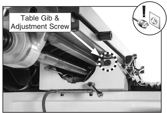
Figure 79. Table gib and adjustment screw underneath left side of table.
