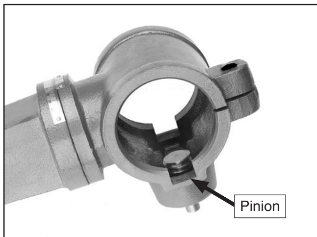
Figure 13. Pinion correctly installed in table support.
