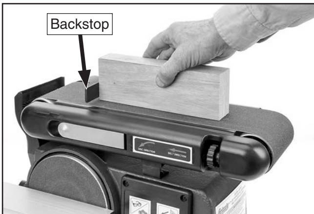
Figure 19. Horizontal belt sanding.
