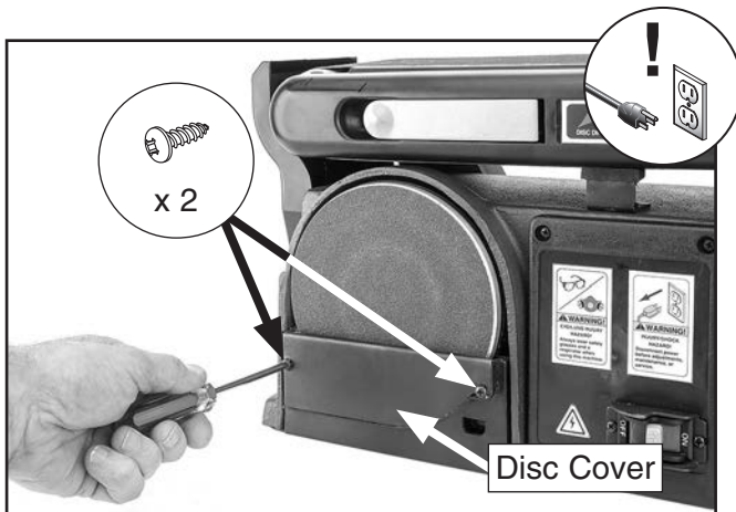
Figure 23. Removing disc cover.
