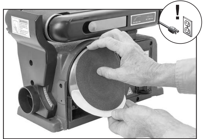
Figure 24. Installing sanding disc.
