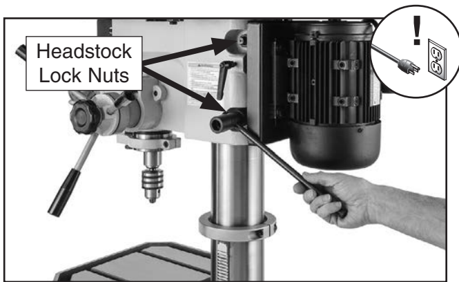
Figure 19. Loosening headstock lock nuts in order to adjust headstock position.
