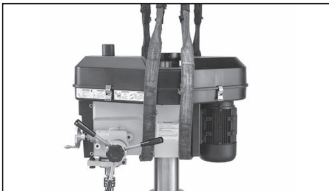
Figure 8. Lifting slings properly wrapped around headstock and positioned to avoid damage to belt cover while lifting.
