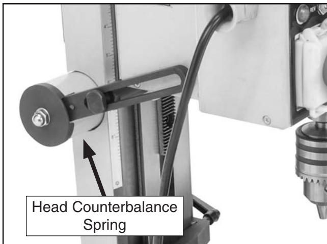
Figure 40. Location of head counterbalance spring.
