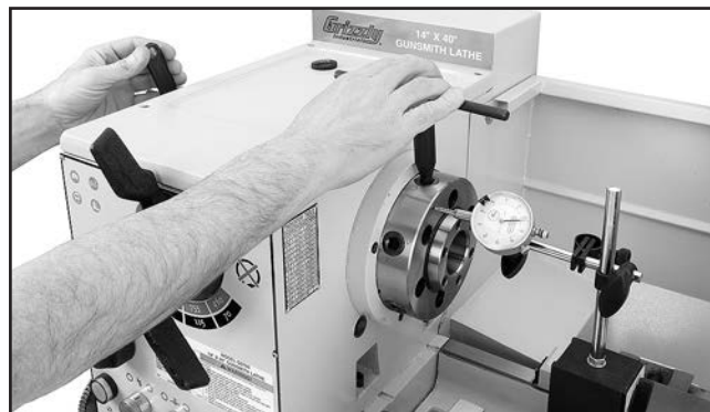
Figure 145. Adjusting spindle bearings.
