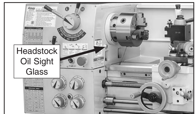
Figure 114. Location of headstock oil sight glass.
