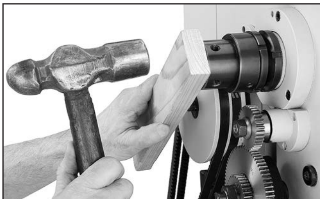
Figure 143. Unseating spindle bearings to introduce spindle end-play.
