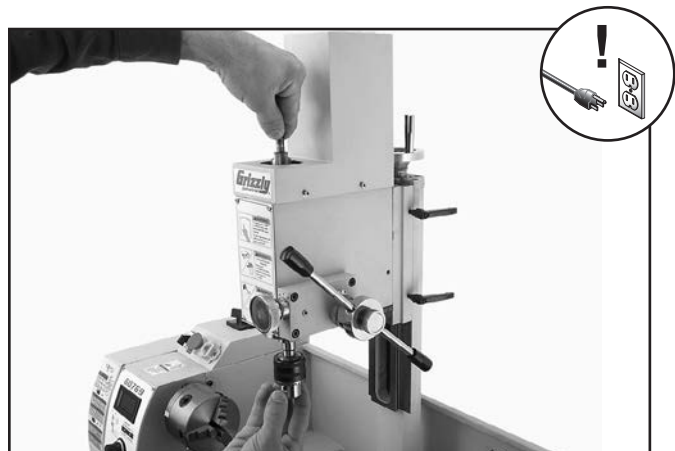
Figure 112. Threading drawbar into tooling.
