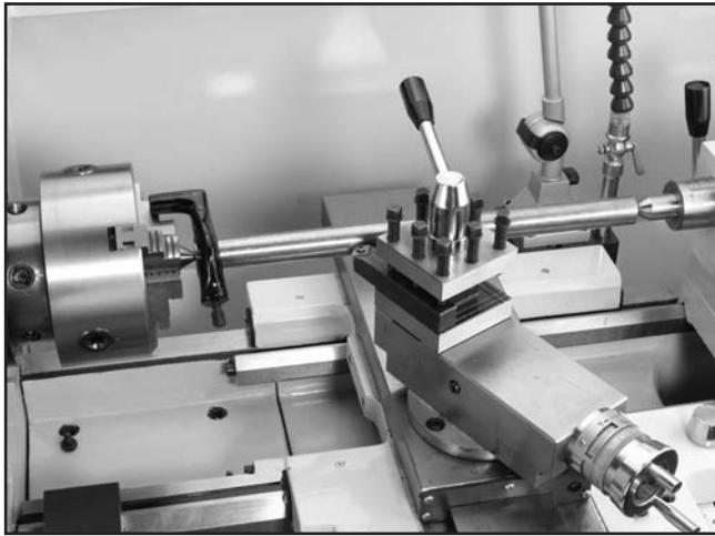
Figure 40. Example of stock mounted between the centers.
