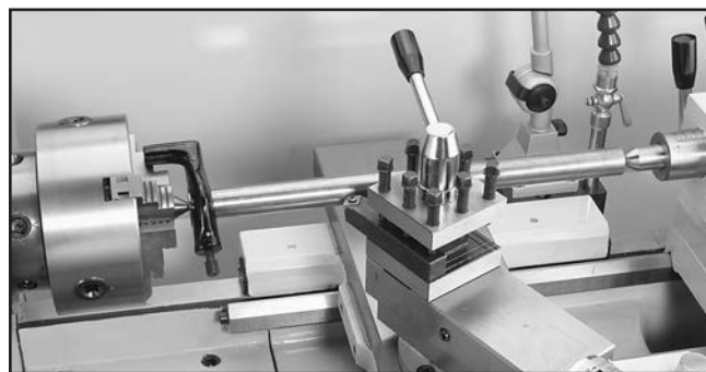
Figure 46. Example photo of a workpiece mounted between two centers.
