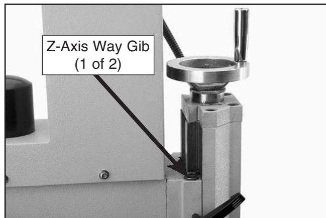
Figure 147. Location of top Z-axis way gib.
