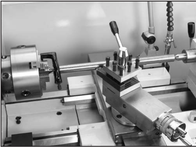
Figure 40. Example of stock mounted between the centers.
