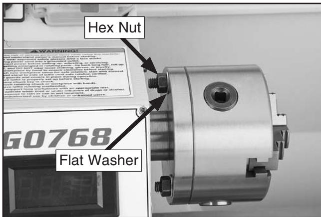
Figure 26. Chuck secured against backplate.
