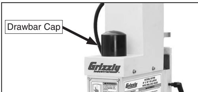
Figure 111. Location of drawbar cap.
