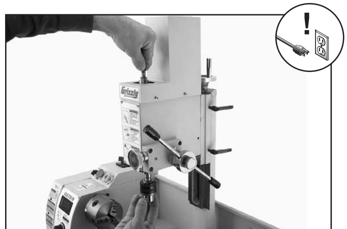
Figure 112. Threading drawbar into tooling.
