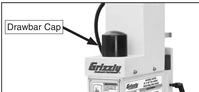
Figure 111. Location of drawbar cap.
