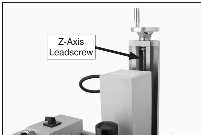
Figure 137. Z-axis leadscrew location.
