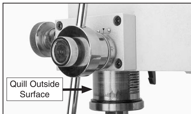
Figure 135. Outside surface of quill.
