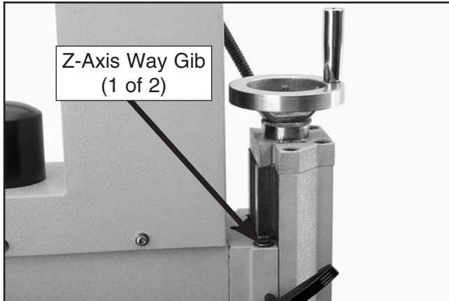
Figure 147. Location of top Z-axis way gib.
