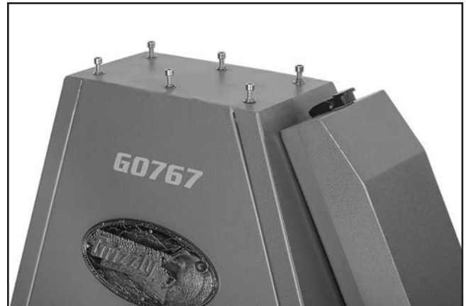
Figure 9. Cap screws on top of base.
