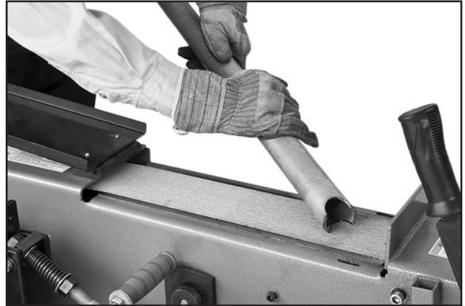
Figure 34. Tube positioned for deburring.
