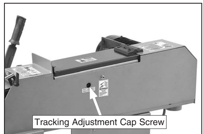
Figure 26. Location of tracking adjustment cap screw.
