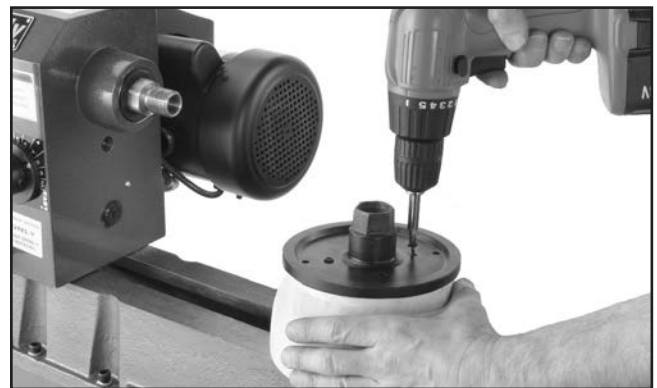
Figure 40. Typical attachment of faceplate to workpiece.
