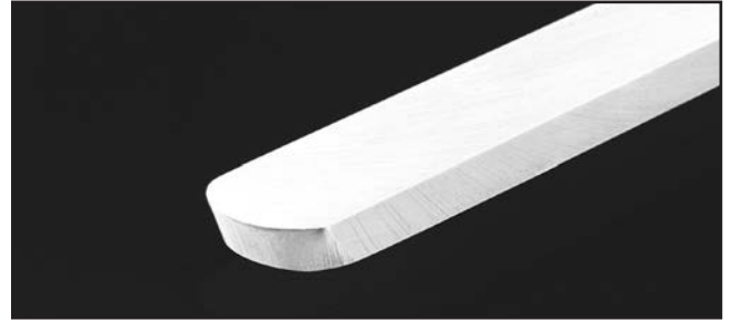
Figure 46. Example of a round nose scraper.
