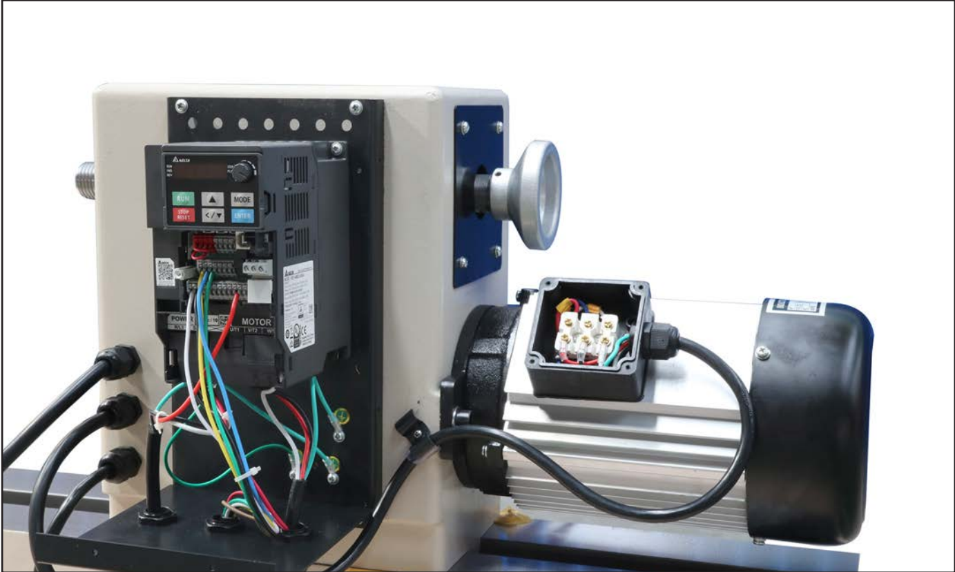
Figure 62. Inverter box and motor box locations.
