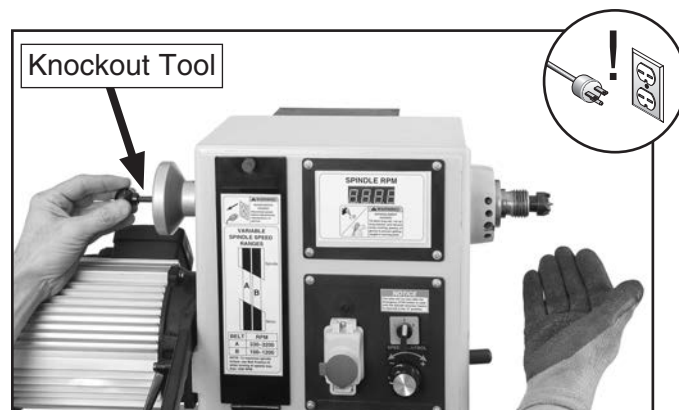
Figure 23. Removing the headstock center.
