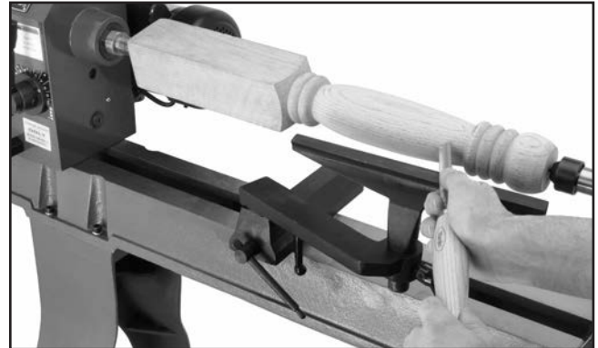
Figure 35. Typical spindle turning operation.
