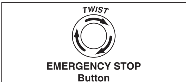
Figure 12. Twisting EMERGENCY STOP button to reset it.
