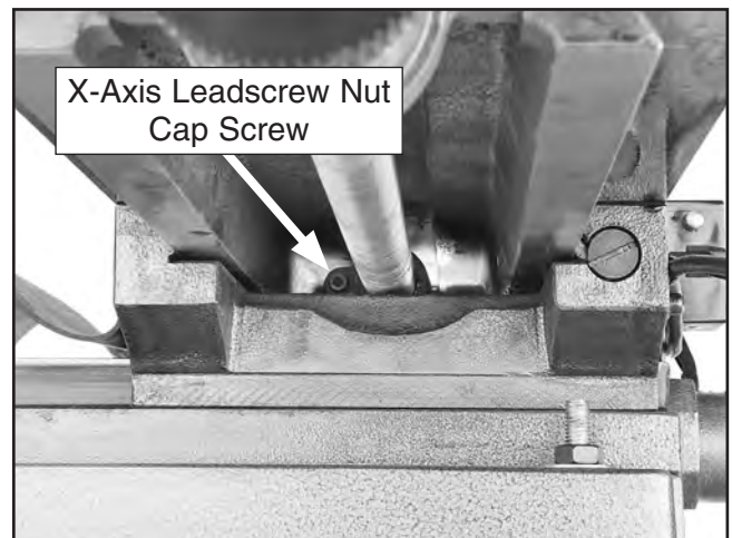
Figure 47. X-axis leadscrew nut adjusting cap screw.
