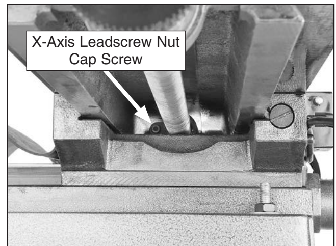
Figure 45. Example of X-axis leadscrew nut cap screw for adjusting backlash.
