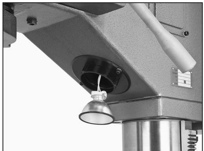
Figure 43. Work lamp wiring.
