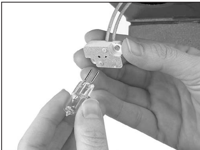
Figure 38. Work lamp bulb replacement.
