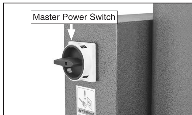
Figure 10. Master power switch.
