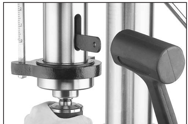
Figure 17. Using drift key to remove arbor.
