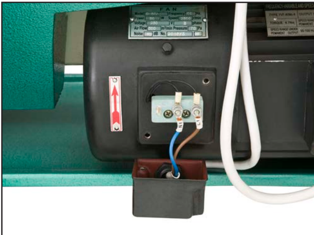
Figure 116. Left motor junction box.
