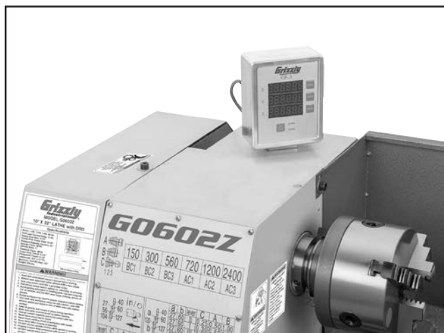
Figure 9. DRO magnetically mounted on lathe headstock.
