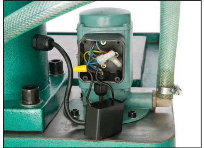
Figure 55. Coolant pump wiring.
