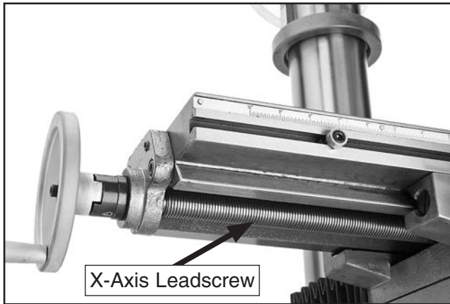
Figure 40. X-axis leadscrew location.
