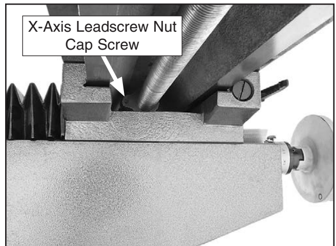
Figure 47. Location of X-axis leadscrew nut for adjusting backlash.
