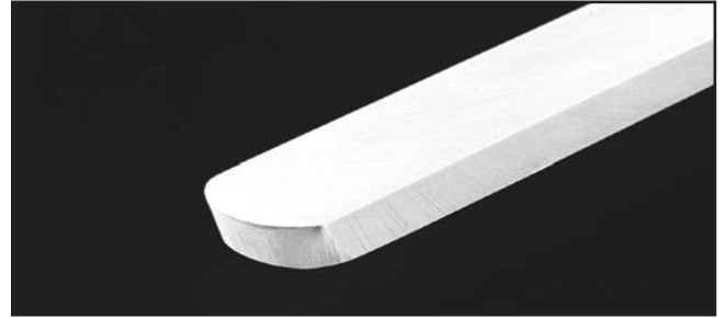
Figure 49. Example of a round nose scraper.
