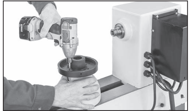
Figure 43. Typical attachment of faceplate to workpiece.
