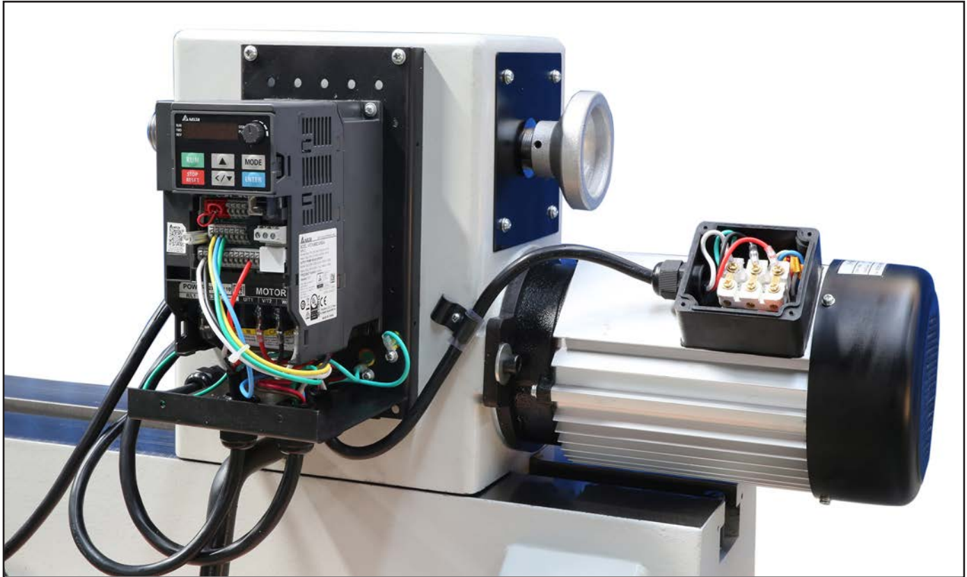
Figure 65. Inverter box and motor box locations.
