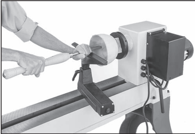
Figure 42. Typical faceplate turning operation.
