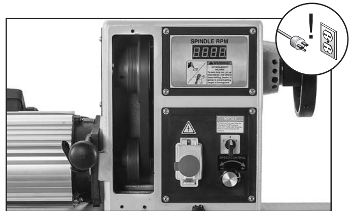
Figure 32. Belt access panel removed.
