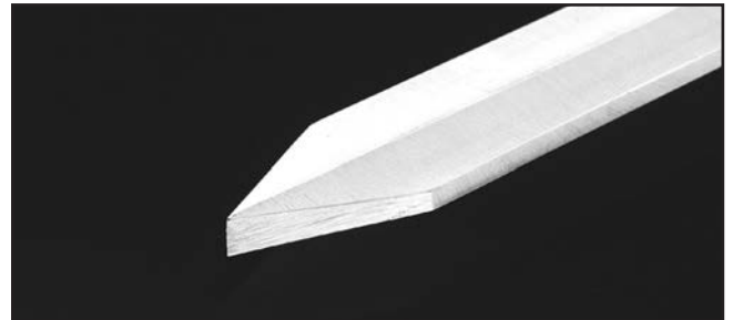
Figure 50. Example of a parting tool.
