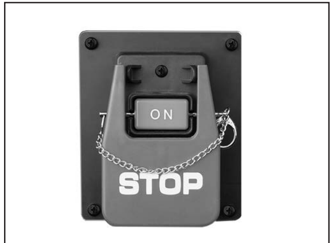
Figure 23. Switch disabling pin installed.
