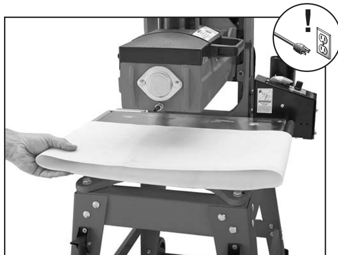
Figure 40. Removing the conveyor belt.
