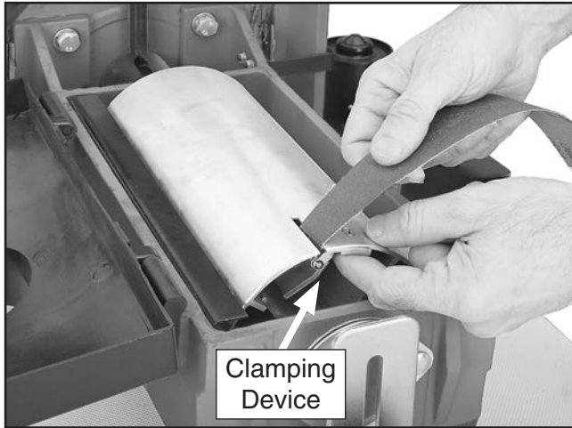
Figure 19. Releasing the clamping device on the left side of the drum.
