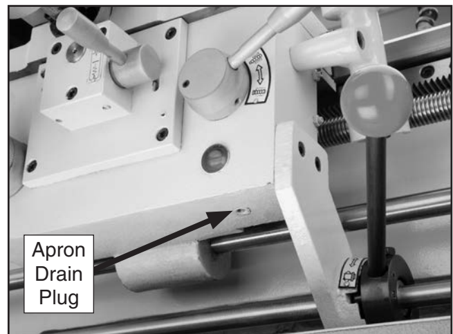
Figure 85. Apron drain plug.
