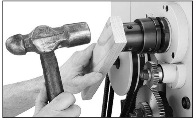
Figure 101. Un-seating spindle bearings to introduce spindle end-play.
