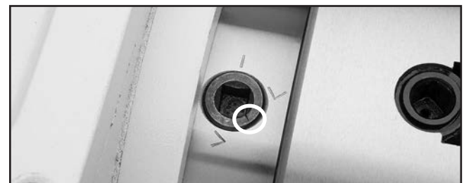
Figure 22. Cam-lock in the locked position.
