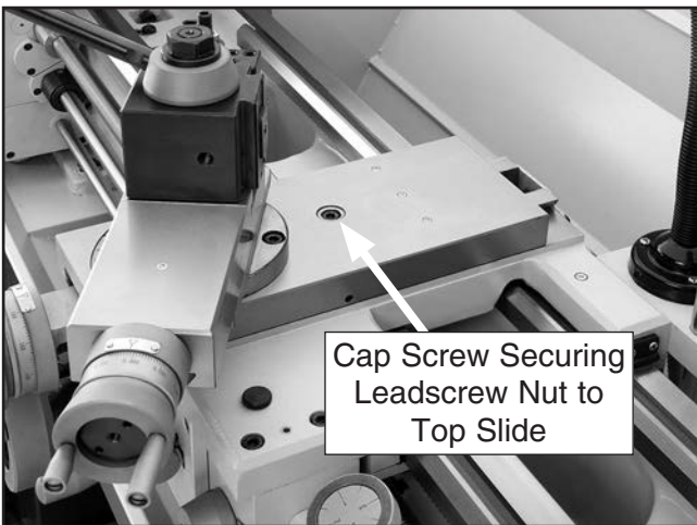
Figure 93. Location of cap screw that secures the leadscrew nut.
