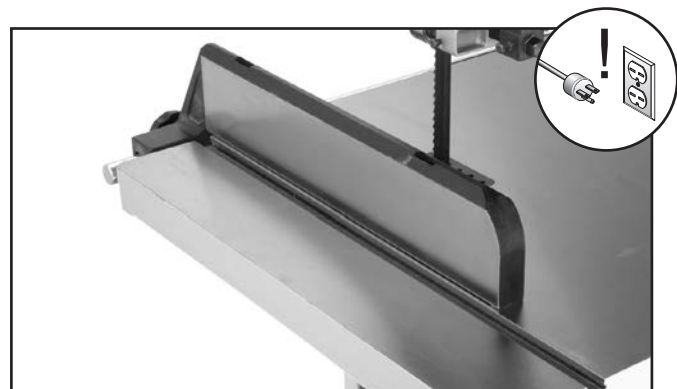
Figure 37. Fence even with the miter slot.
