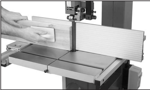
Figure 55. Example of resawing lumber.
