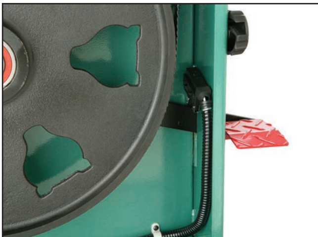
Figure 91. Brake switch wiring.
