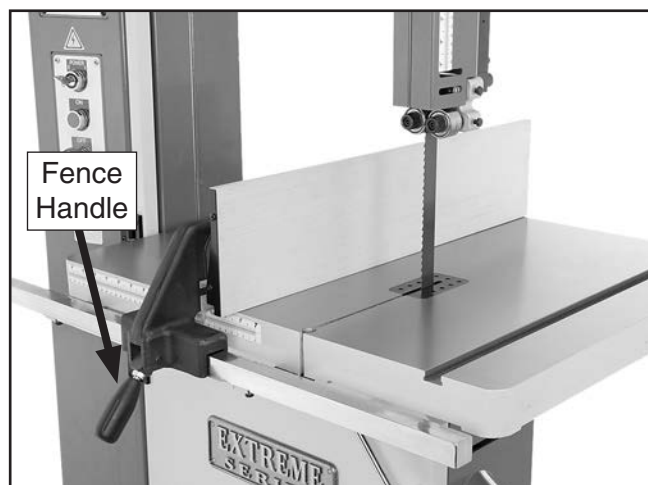
Figure 12. Fence assembly mounted on the fence rail.
