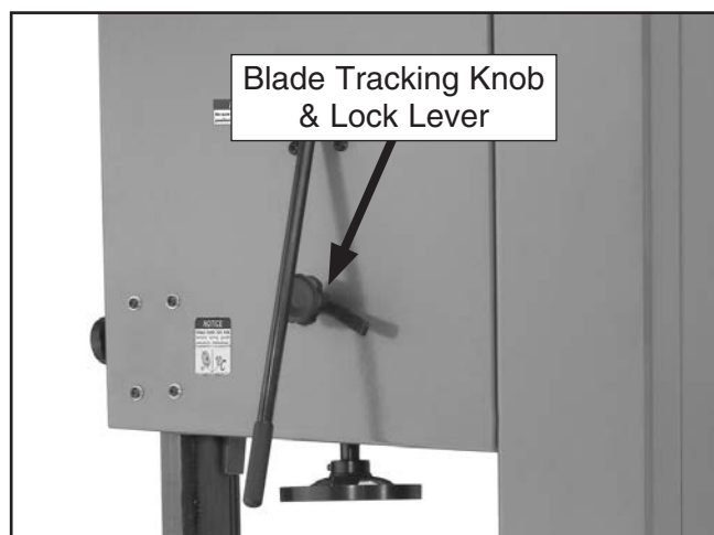
Figure 16. Blade tracking knob and lock lever.
