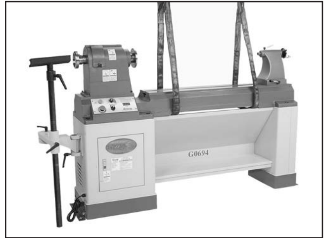
Figure 9. Lifting straps positioned to lift the lathe.
