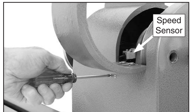
Figure 68. Reinstalling speed sensor.
