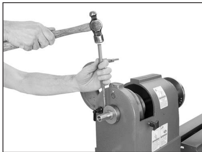
Figure 58. Unseating outboard spanner nut.
