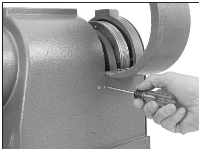
Figure 60. Removing speed sensor screws.
