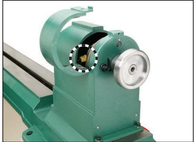
Figure 3. Tachometer sensor location.
