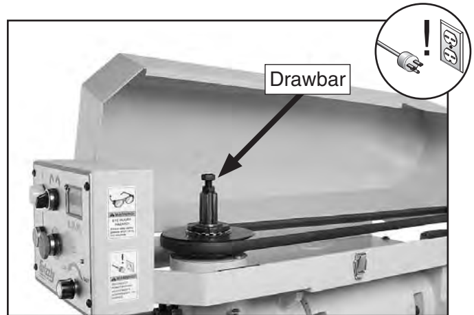
Figure 26. Drawbar inserted through the top of the spindle.
