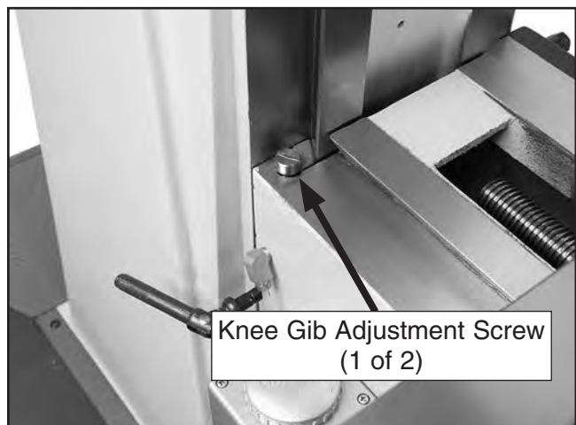
Figure 43. Knee gib adjustment screw (1 of 2).
