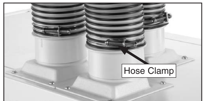
Figure 17. Example of dust collection hose attached to dust port.
