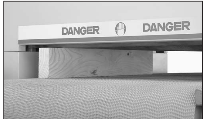
Figure 20. Checking pressure roller height.
