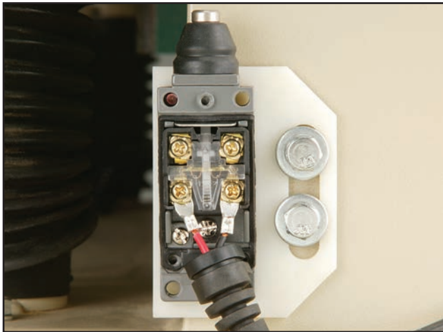
Figure 96. Lower table limit switch.
