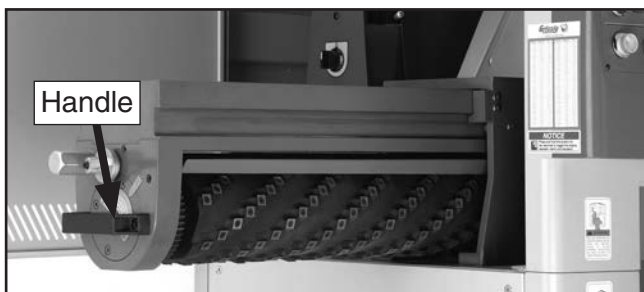
Figure 11. Spiral cutterhead access.
