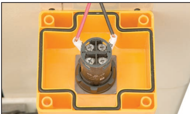
Figure 89. Rear emergency stop button wiring.
