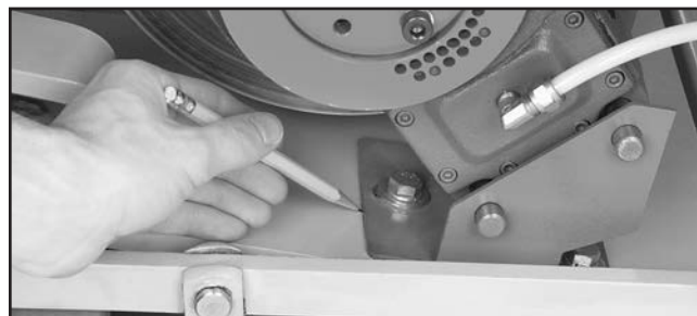
Figure 71. Marking caliper assembly location.
