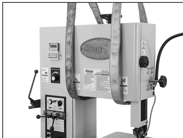
Figure 7. Lifting straps positioned on bandsaw.
