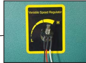
Figure 54. Variable speed dial wiring.
