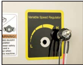
Figure 2. Variable speed dial wiring.
