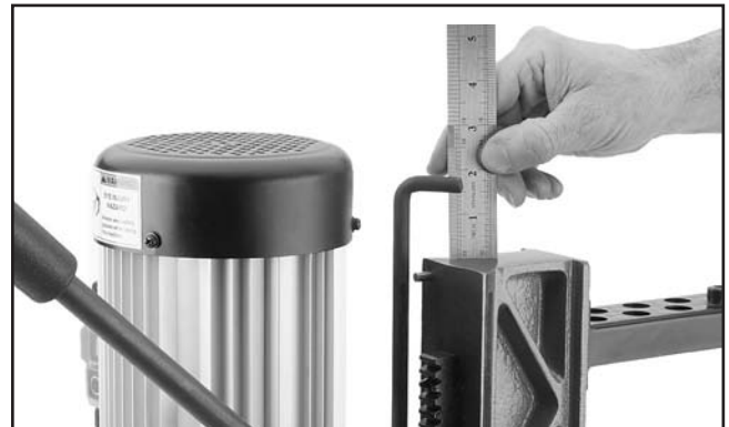
Figure 22. Adjusting depth stop using ruler.
