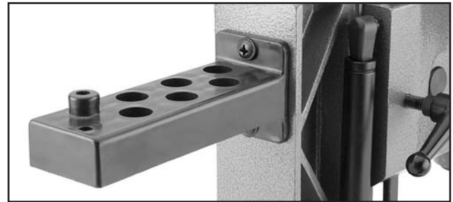
Figure 13. Tool storage rack installed.
