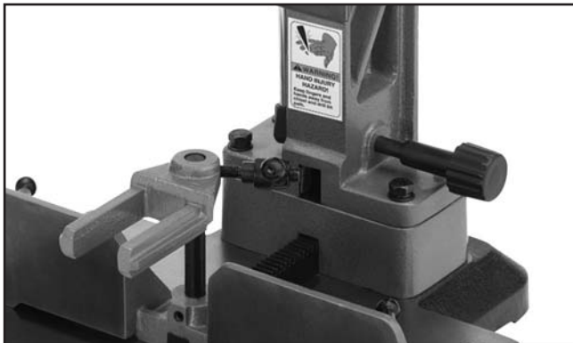
Figure 16. Extension block installed.
