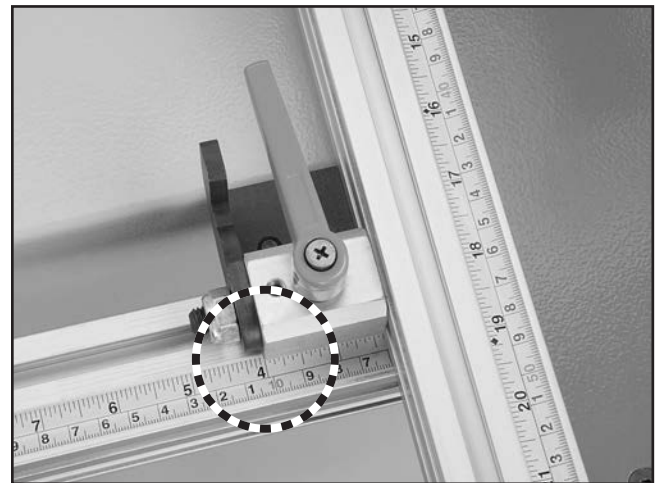
Figure 23. Distance of 4" of the longitudinal fence from boring bit centers, as read on the cross fence scale.
