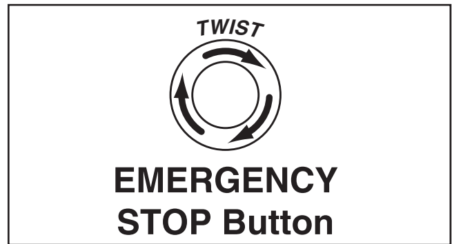
Figure 15. Resetting the switch.
